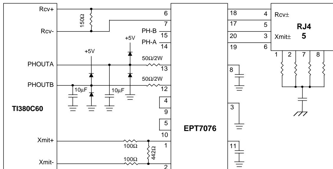
Notes : 1. Pins 15 & 14 are left unconnected. Applications vary. Your system may have a phantom drive return detection circuit needing pins 15 & 14 to be connected separately or together, can be taken to ground via an inductor.
