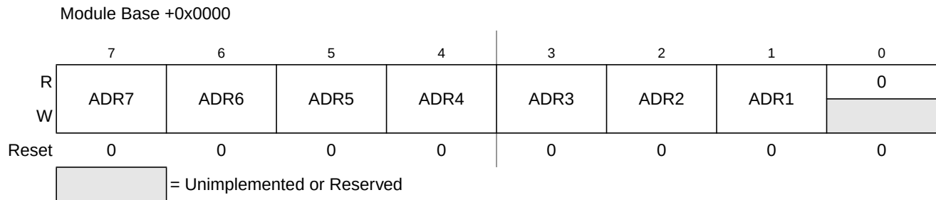
Figure 10-3. IIC Bus Address Register (IBAD)
