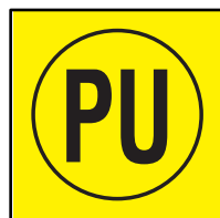
PESC*-PU Protective conductor - no earth
