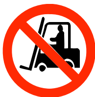
PESV-*12 No access for industrial vehicles
