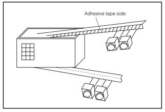
Drawing-out can be done from top or bottom of an inner carton.
