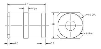
DIMENSIONS: MILLIMETERS  $\label{eq:dimension} \mbox{DIMENSION TOLERANCE: } .X \pm 0.25$
