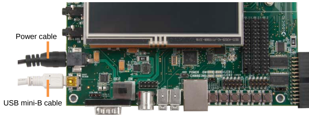
Figure 2.2: Connect USB Mini-B Cable
