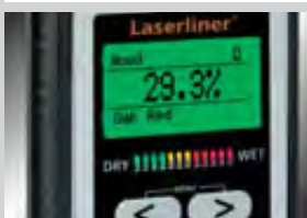
12-position wet/dry LED indicator
