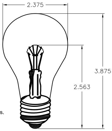
Rough service bulbs are made with strong and well-supported filaments to resist vibrations, shocks, and bumps.
