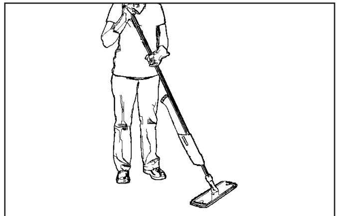
Figure 5. Applying floor finish with Flat Mop (optional).
