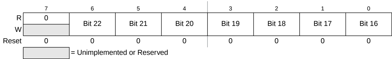
Figure 20-15. Debug Comparator Address High Register (DBGXAH)
