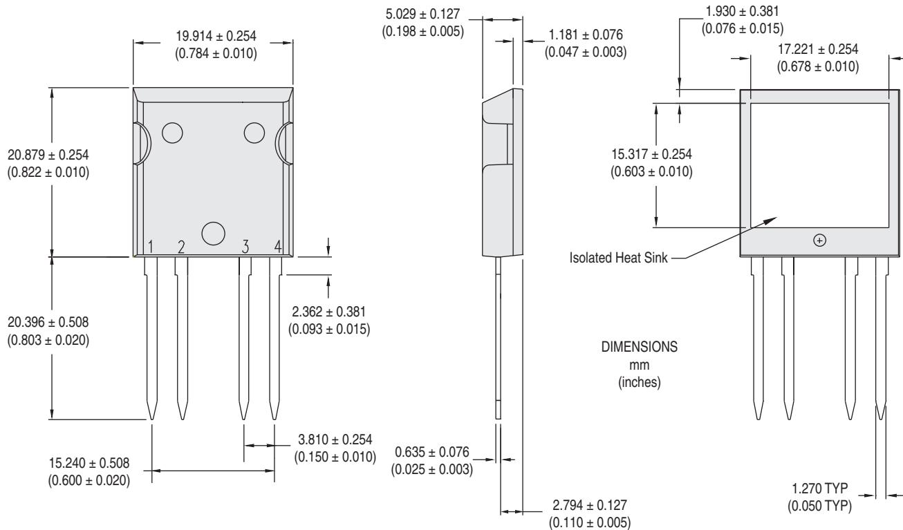
NOTE: Back-side heat sink meets 2500V<sub>rms</sub> isolation to the pins.
