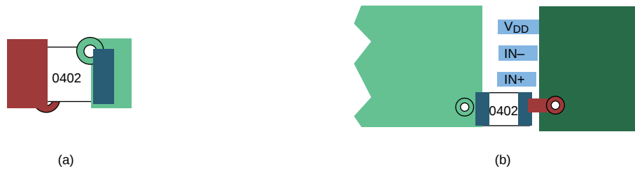
Figure 33. Typical Decoupling Capacitor Layouts
