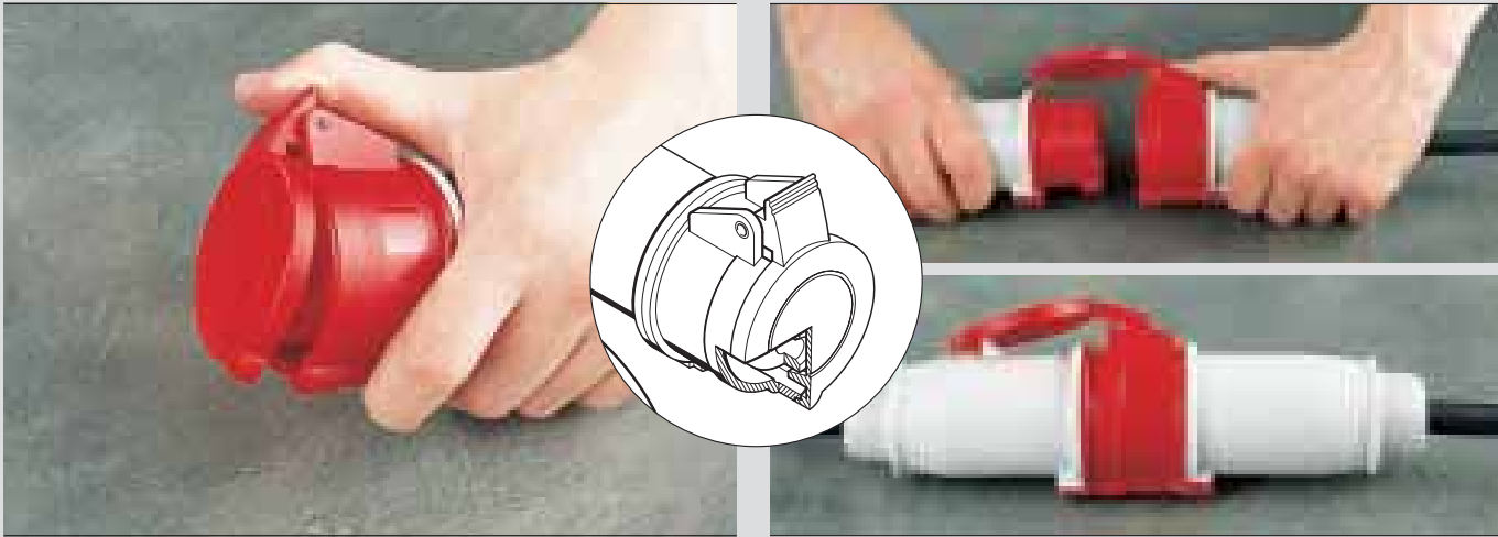
A wing on the lid assists one-handed opening. Splash-proof protection (IP44) is assured by the two inclined surfaces on the lid and on the insert. These surfaces also assist self-centring of the lid.
