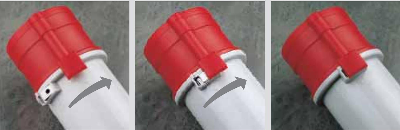
The spring on the side of the grip holds it fast against the insert. By twisting the assembly, the spring snaps into its housing.
