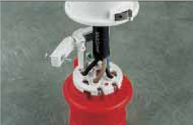
The cable clamp is located inside the housing to protect it from damage. The cable is clamped by tightening one single screw using a screwdriver for either single-slotted or cross-slotted screws. To assist wiring operations, the cable clamp is equipped with a “catch” to keep it open and to leave room for the hands when installing.
