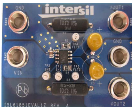
FIGURE 32B. ISL61851EVAL1Z BOARD PHOTO
