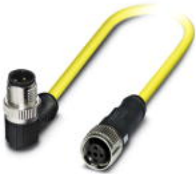
Sensor/actuator cable, 3-position, PVC, Plug angled M12 SPEEDCON, A-coded, on Socket straight M12 SPEEDCON, A-coded, cable length: 3 m
