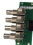
Video input daughter board With 4 x BNC connectors
