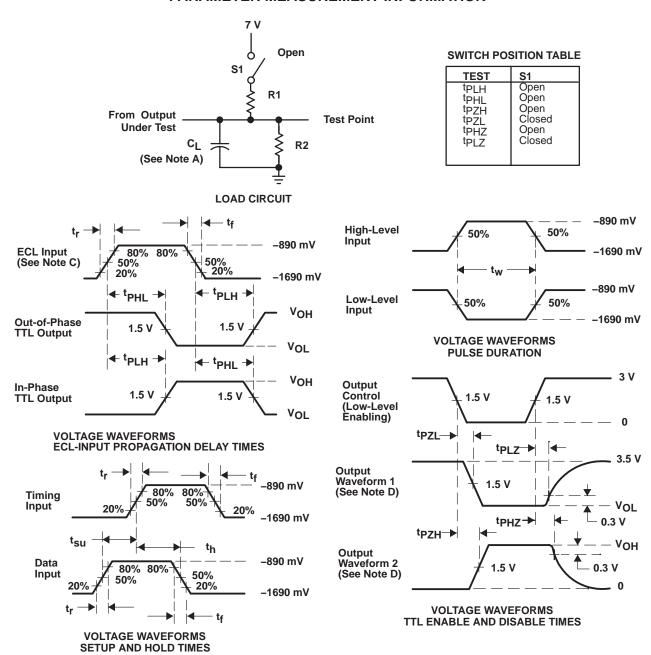
NOTES: A.C<sub>I</sub> includes probe and jig capacitance.
