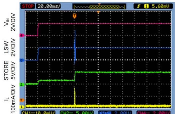
Startup : Circuit A with R_{IN}=10\Omega V_{IN}=2V , STORE=5V, I_{STORE}=0.5\mu A
