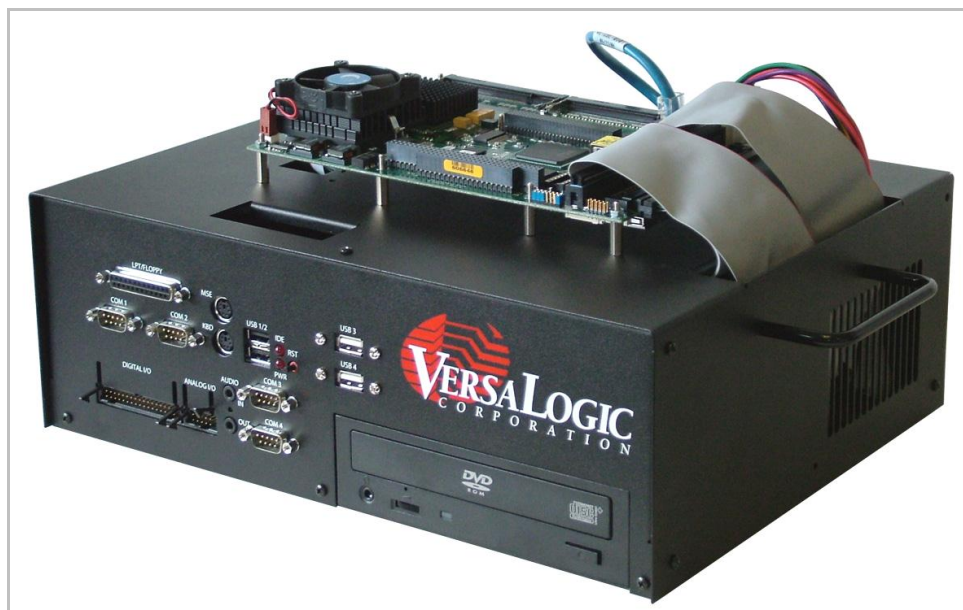
Figure 10. Example EBX Board Installation
