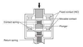
Conforms to EN60947-5-1 Direct Opening Operation →
