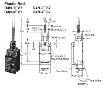
**Note: 1.** Unless otherwise specified, a tolerance of  $\pm 0.4$  mm applies to all dimensions.
