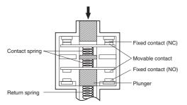
Conforms to EN60947-5-1 Direct Opening Operation ←
