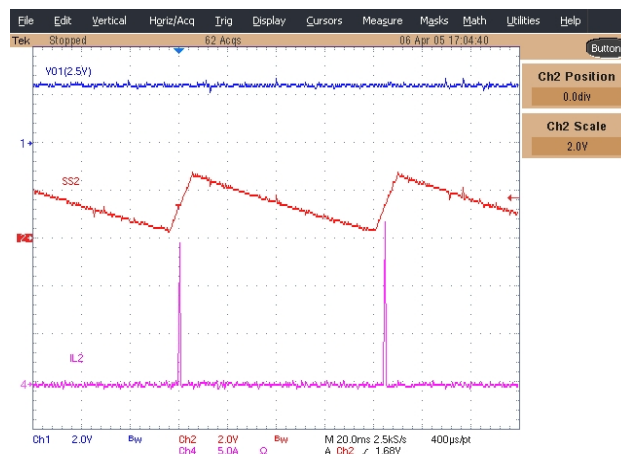
Figure 30 - 1.8V output shorted Ch1: Vo1, Ch2: SS2, Ch3: Inductor Current
