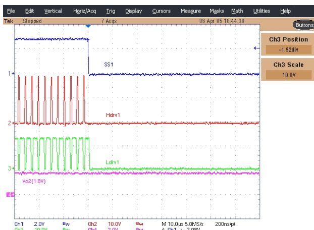
Figure 33 - SS1 pin shorted to Gnd Ch1: SS1, Ch2: Hdrv1, Ch3: Ldrv1, Ch4: Vo2
