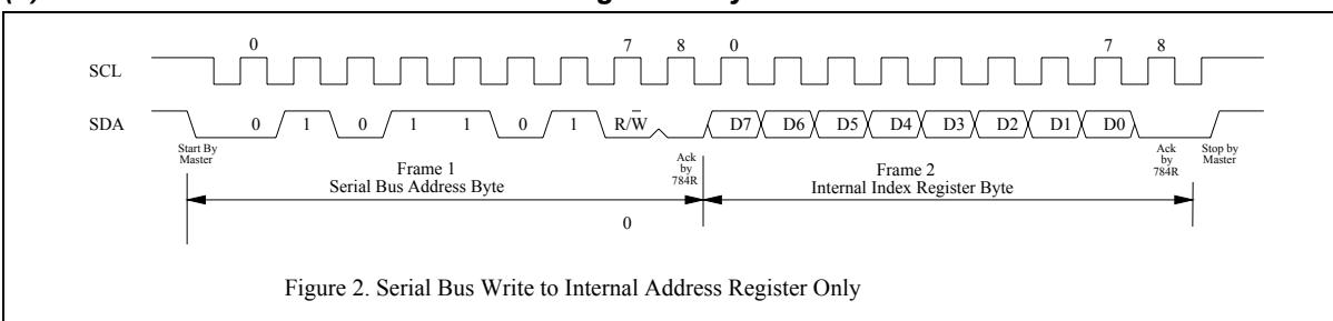
Figure 2. Serial Bus Write to Internal Address Register Only
