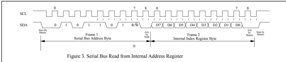
**6.2.2 The serial bus timing of the temperature CPUT1 and CPUT2 is shown as follow:**
