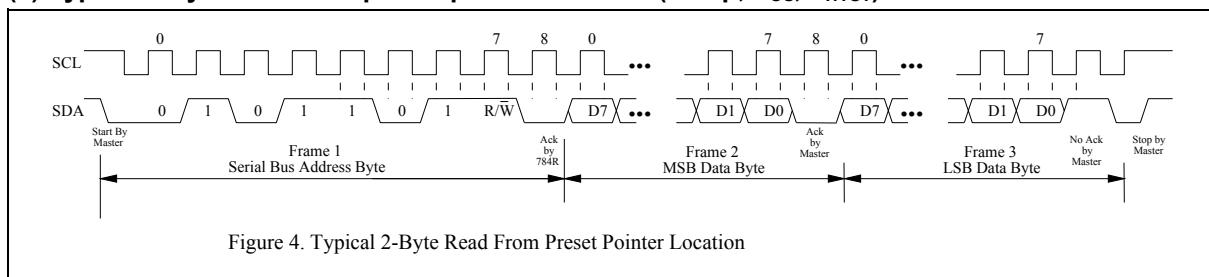
**(b) Typical pointer set followed by immediate read for 2-byte register (Temp, Tos, THYST)**
