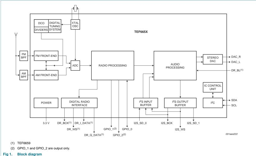
**DSP-based radio tuner one-chip**
