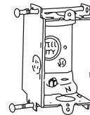
A257-25 With nails slanted for easy drive-in
