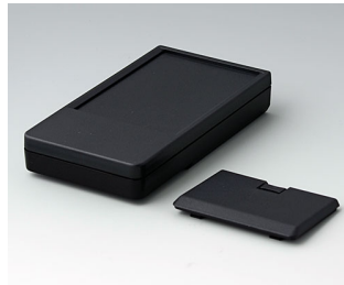
A9072129 DATEC-POCKET-BOX L ABS (UL 94 HB) black RAL 9005 4.72"x2.56"x0.87" IP 41
