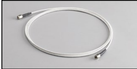
CA-404B: 2m (6.5 ft) RG188 coax cable terminated with an SMA male plug on each end, 50Ω impedance.
