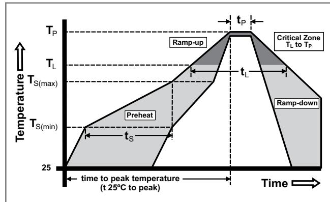
**Soldering Parameters - Wave Soldering (Thru-Hole Devices)**
