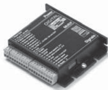
DECV 50/5 4-Q-EC Amplifier 4-quadrant controller for brushless EC motors with Hall sensors up to 250 watts.
