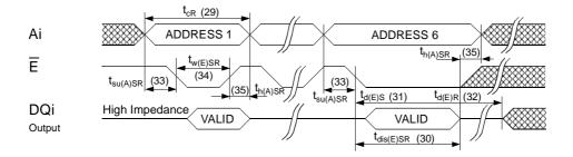
w:  $\overline{\mathsf{E}}$  must be used to clock in the address sequence for the Software controlled STORE and RECALL cycles.
