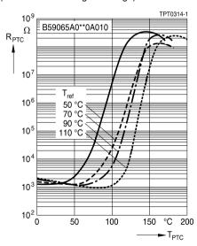
PTC resistance  $R_{\text{PTC}}$  versus PTC temperature T<sub>PTC</sub> (measured at low signal voltage)
