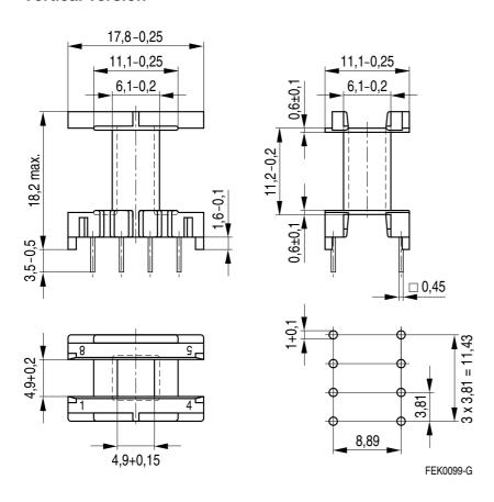
Hole arrangement View in mounting direction
