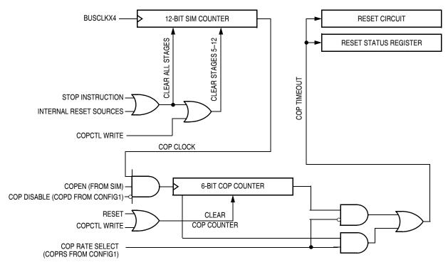
Figure 6-1. COP Block Diagram
