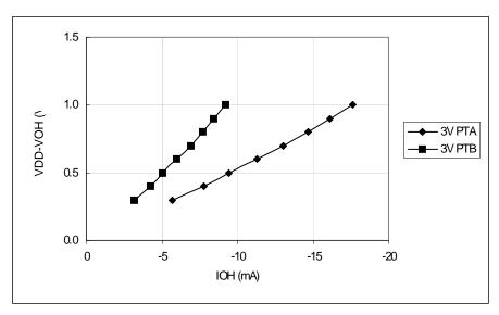
Figure 16-5. Typical 3-Volt Output High Voltage versus Output High Current (25•C)
