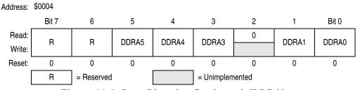
Figure 12-2. Data Direction Register A (DDRA)
