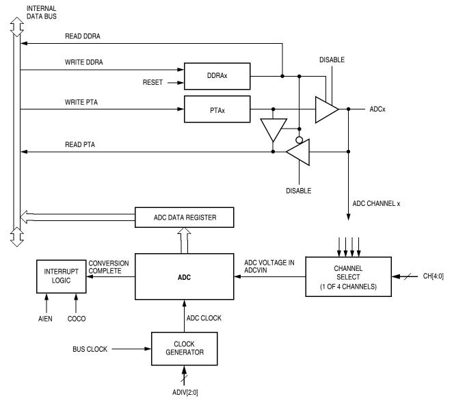
Figure 3-2. ADC Block Diagram
