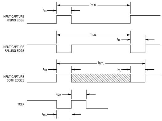
Figure 16-11. Timer Input Timing
