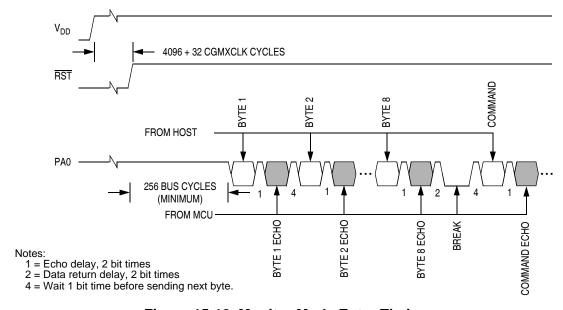
Figure 15-18. Monitor Mode Entry Timing
