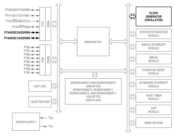
RST, IRQ: Pins have internal (about 30K Ohms) pull up
