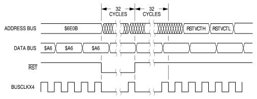
Figure 13-16. Wait Recovery from Internal Reset
