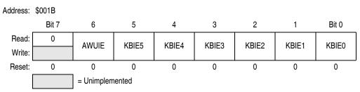
Figure 9-4. Keyboard Interrupt Enable Register (KBIER)
