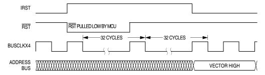
Figure 13-4. Internal Reset Timing
