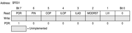
Figure 13-19. SIM Reset Status Register (SRSR)
