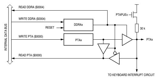
Figure 12-3. Port A I/O Circuit
