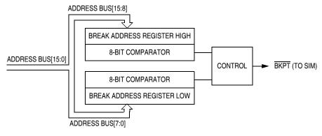
Figure 15-2. Break Module Block Diagram
