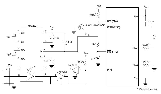
Figure 15-10. Monitor Mode Circuit (External Clock, with High Voltage)
