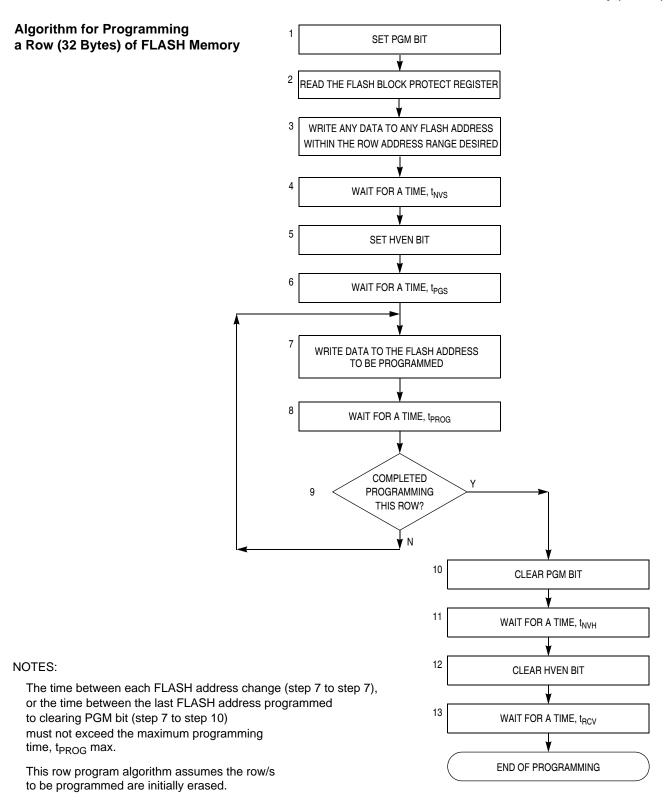
Figure 2-4. FLASH Programming Flowchart
