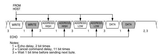
Figure 15-16. Write Transaction
