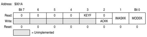
Figure 9-3. Keyboard Status and Control Register (KBSCR)
