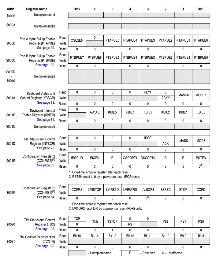
Figure 2-2. Control, Status, and Data Registers (Sheet 2 of 5)
