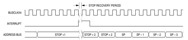
Figure 13-18. Stop Mode Recovery from Interrupt
