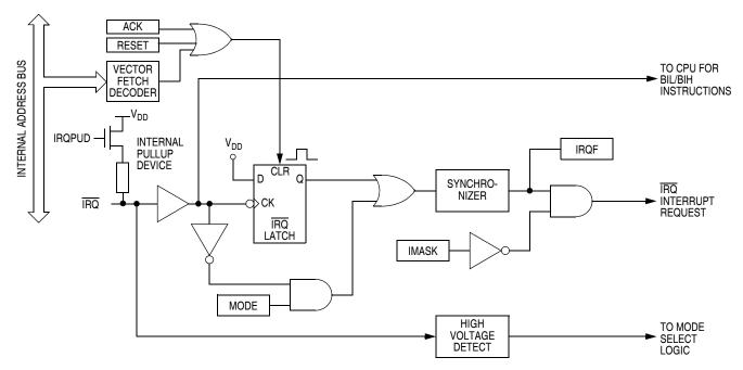
Figure 8-2. IRQ Module Block Diagram
