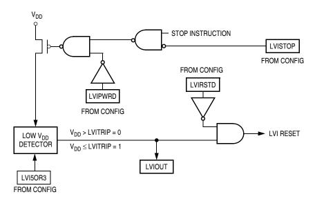
Figure 10-1. LVI Module Block Diagram
