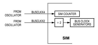
Figure 13-2. SIM Clock Signals
