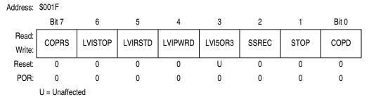
Figure 5-2. Configuration Register 1 (CONFIG1)
