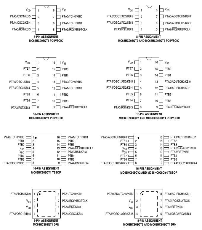
Figure 1-2. MCU Pin Assignments
