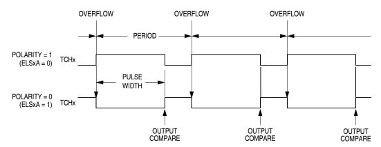
Figure 14-3. PWM Period and Pulse Width
