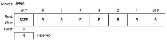
Figure 13-20. Break Flag Control Register (BFCR)
