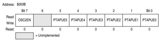
Figure 12-4. Port A Input Pullup Enable Register (PTAPUE)
