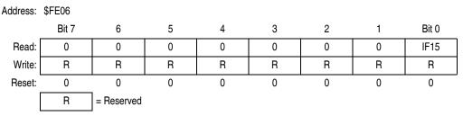
Figure 13-13. Interrupt Status Register 3 (INT3)
