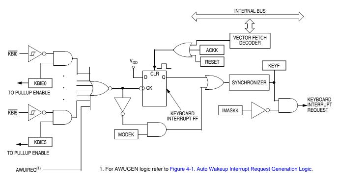
Figure 9-2. Keyboard Interrupt Block Diagram
