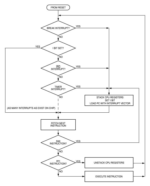
Figure 13-7. Interrupt Processing
