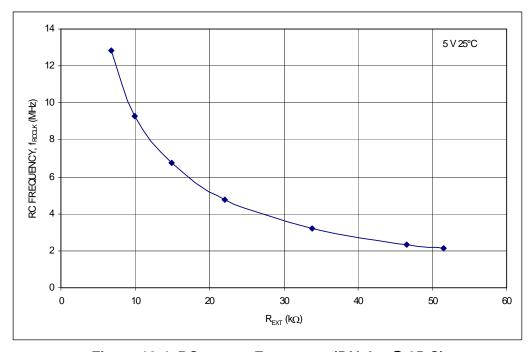
Figure 16-4. RC versus Frequency (5 Volts @ 25•C)
