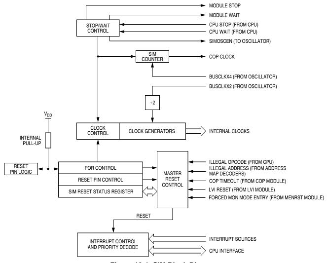
Figure 13-1. SIM Block Diagram
