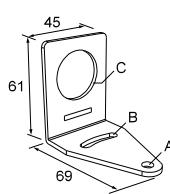
**Hole center spacing:** A to B=40**Hole size:** A=ø 6.3, B= 27.1 x 6.3, C=ø 30.5**SMB30FA**
