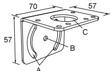
**Hole center spacing:** A = 51, A to B = 25.4**Hole size:** A = 42.6 x 7, B = ø 6.4, C = ø 30.1**SMBAMS30P**
