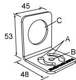
**Hole center spacing:** A=26.0, A to B=13.0**Hole size:** A=26.8 x 7.0, B=ø 6.5, C=ø 31.0**SMB30SC**
