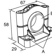
**Hole center spacing:** A=ø 50.8**Hole size:** A=ø 7.0, B=ø 30.0**LMB Sealed Right-Angle Bracket**
