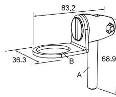
**Bolt thread:** SMB30FA, A= 3/8 - 16 x 2 in; SMB30FAM10, A= M10 - 1.5 x 50**Hole size:** B= ø 30.1**SMB30MM**
