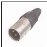
30-630-SL-3 3 pin 30-630-SL-4 4 pin 30-630-SL-5 5 pin Silver inline male XLR plug. .15" to .3" cable opening. No tools required for assembly or disassembly. 4 piece construction. Internal compression style cable strain relief.
