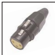
30-631-BK-3 3 pin 30-631-BK-4 4 pin 30-631-BK-5 5 pin Black inline female XLR plug. .15" to .3" cable opening. No tools required for assembly or disassembly. 4 piece construction. Internal compression style cable strain relief.
