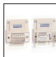
30-593 VGA to MAC adapter, 6 position Dip Switch For connecting Apple 15 pin (2 rows) to 15 pin (3 rows) D sub connectors. Supports Apple standard display modes including 13" color (640x480) 16" (832x- 624) 21" (1152x870). Dip switch selectable for different display modes.
