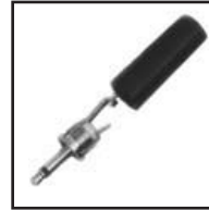
30-423A 2.5 mm sub-mini Audio Plug with plastic grip, 2 cond. Improved solder points. 7/16" plug length. .15" cable opening.
