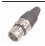
30-631-SL-3 3 pin 30-631-SL-4 4 pin 30-631-SL-5 5 pin Silver inline female XLR plug. .15" to .3" cable opening. No tools required for assembly or disassembly. 4 piece construction. Internal compression style cable strain relief.
