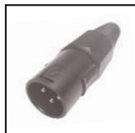
30-630-BK-3 3 pin 30-630-BK-4 4 pin 30-630-BK-5 5 pin Black inline male XLR plug. .15" to .3" cable opening. No tools required for assembly or disassembly. 4 piece construction. Internal compression style cable strain relief.
