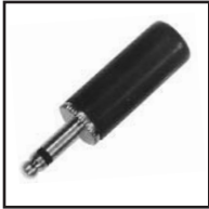
30-416-BK black 30-416-RD red 3.5 mm mono Audio Plug with solder terminals & cable clamp. .18" cable opening.
