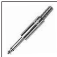
30-404 Nickel 30-404G Gold 1/4" Mono Audio Plug with strain relief. .28" cable opening.
