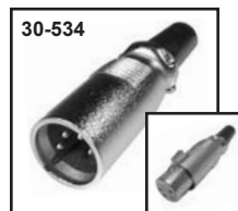
30-534 Silver 30-534-BK Black 4-pin XLR inline male plug in silver or black. 30-535 Silver 30-535-BK Black 4-pin XLR inline female jack in silver or black. .25" cable opening
