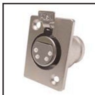
30-523-SL-4 4 pin 30-523-SL-5 5 pin 4 or 5 pin female XLR chassis jack mounts in .9375" or \frac{15}{16} " hole size.
