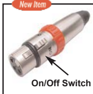
30-638 3-Pin XLR inline female with labeled on/off switch. Shorts pins 2 & 3 to mute signal voltage with plastic noiseless switch. Gold plated contacts.
