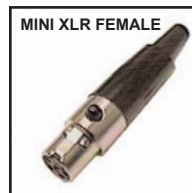
30-641-3 3 pin 30-641-4 4 pin 30-641-5 5 pin 30-641-6 6 pin Inline female MINI XLR jack. Also available with short boot. Cable opening .13"-.17"
