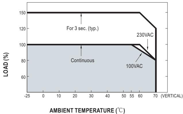
**■ Output derating VS input voltage**
