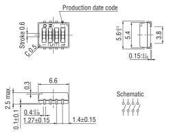
Unless otherwise specified, tolerance: ± 0.3 (Unit: mm)
