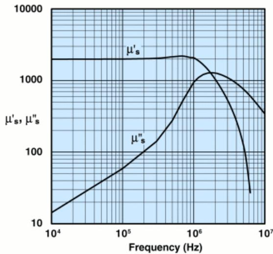
Measured on an 18/10/6mm toroid
