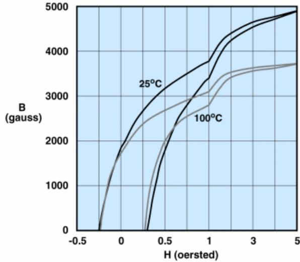
Measured on an 18/10/6mm toroid at 10kHz.
