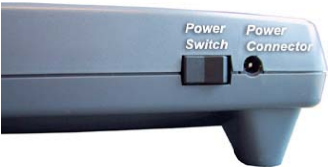
Figure 3-7. Power Switch and Connector
