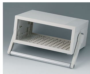
B2211317 MEDITEC D 160, with handle bar ABS (UL 94 HB) off-white RAL 9002 11.42"x7.87"x4.88" IP 40
