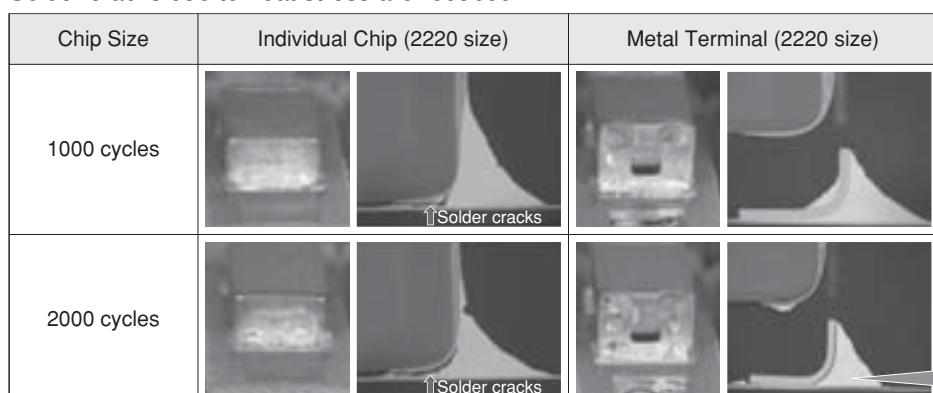
Test Conditions: -55 to +125°C, 5 minutes (liquid phase)
