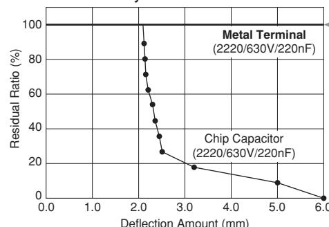
Solder cracks due to heat stress are reduced.
