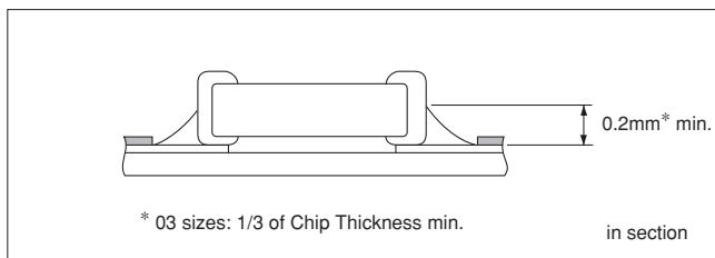
\* 03 sizes: 1/3 of Chip Thickness min.
