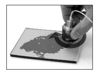
19.9 Once polishing is complete, refer to steps 17.14 through 17.17 on inspecting the connector with the 200X fiber view scope before proceeding to final step.
