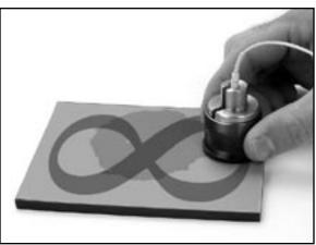
18.10 Leaving the polishing jig assembly positioned on the lapping film, rotate 180 degrees. Perform 3 to 4 additional figure eights.
