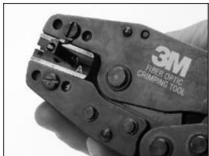
15.4 Using the LC die labeled "B" line up the non-lettered side of the die with the rear of the crimp die and crimp the right half of the crimp ring.
