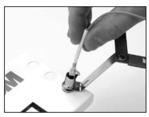
14.2 Remove the connector from the load adapter.
