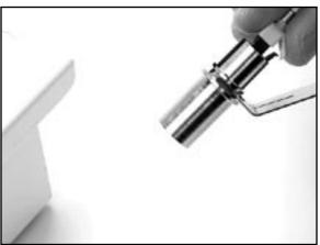
14.3 Using the die labeled "A" with the 3M lettering facing to the left, crimp the metal portion of the sleeve once.
