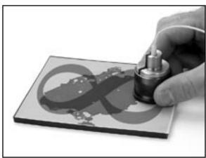
19.8 Leaving polishing jig assembly positioned on the lapping film rotate 180 degrees. Perform 4 additional figure eights.
