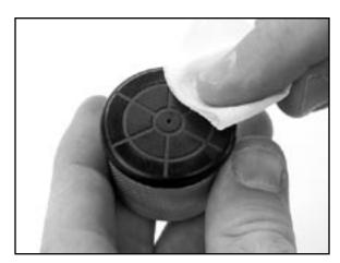
18.9 Place the polishing jig assembly on the wet diamond lapping film. Perform 3 to 4 figure eights.
