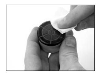
17.8 Place the polishing jig assembly on the lapping film.
