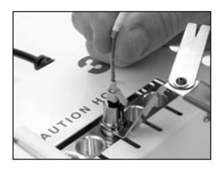
12.2 Maintaining fiber position in connector, push the jacketed fiber into the cable v-slot feature on the load adapter until secure.
