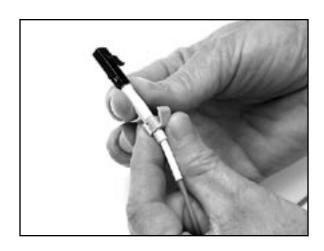
21.3 Taper on the boot will cause the yoke to spread allowing the correct placement at the rear of the connector.
