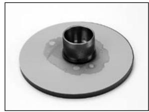
17.9 Place the ferrule in the polishing jig aligning the latch side of the connector with the slot until it stops.
