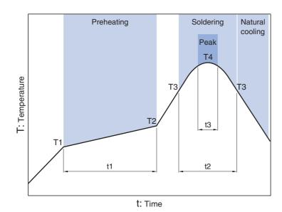
Preheating Soldering Peak Temp. Temp. Temp. Time Time Time T1 T2 Т3 **T4** t3 150°C 180°C 60 to 120s 230°C 30 to 60s 250 to 260°C 10s max.
