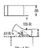
The rocker switches offer a remarkable silicone rubber seal that protects contacts and mechanisms better than conventional seal and boot combinations. The switches resist contaminants such as sand, dust and moisture with both base to frame seal and an actuator seal. **Rated:** 15 A, 125 VAC; 10 A, 250 VAC. **Spade Terminals:** Brass. Concave rocker. Illuminated versions available.
