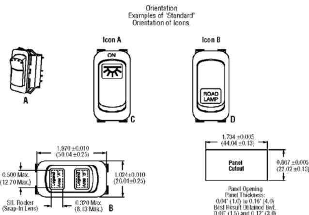
This all new line of rockers offers European styling, ergonomic design with the solid durability you've come to expect from Eaton switches. Rockers and bezels for the NGR series are molded in a soft matte finish. Illuminated and non-illuminated versions are available.
