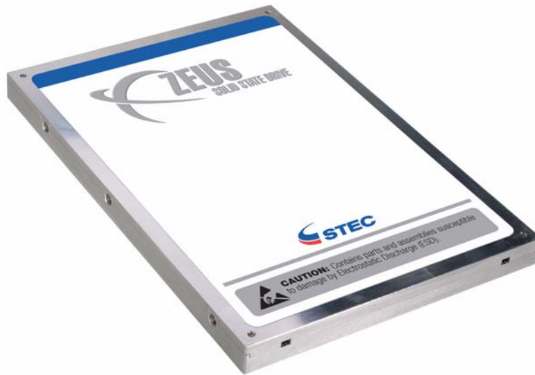
Figure 1. The Zeus 2.5-Inch SATA Solid State Drive
