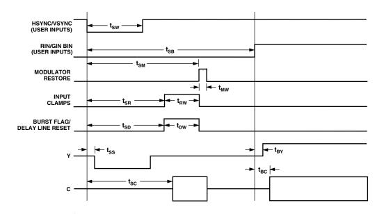
Figure 6. Timing Diagram (Not to Scale)
