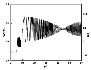
Figure 12. Luminance Sweep with Trap, CV Pin
