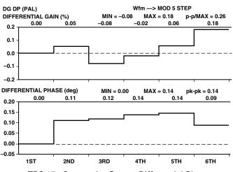
TPC 15. Composite Output Differential Phase and Gain, PAL
