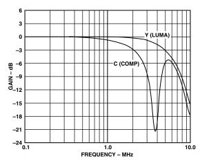
Figure 13. Luminance Frequency Response with NTSC Trap
