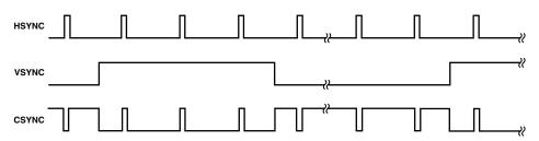
Figure 14. Sync Logic Levels (Equalization and Serration Pulses Not Shown)
