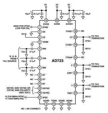
Figure 7. Basic Connection (Using Direct Input Termination)
