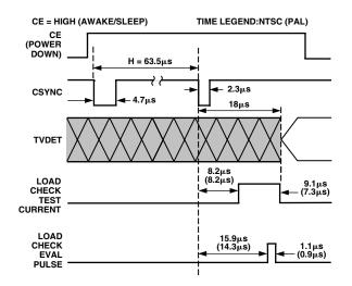
Figure 5. Timing Diagram for Load Check
