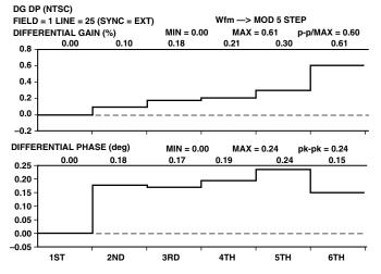
TPC 12. Composite Output Differential Phase and Gain, NTSC
