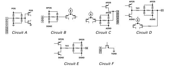
Figure 1. Equivalent Circuits
