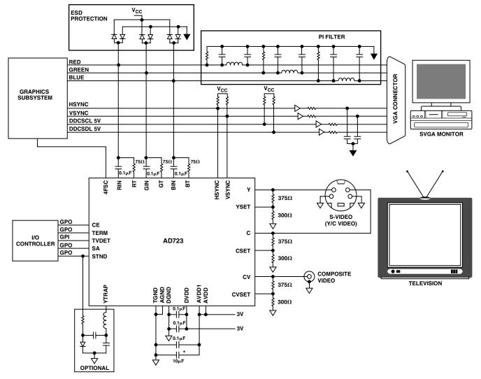
Figure 8. PC Interface (Using Switch Input Termination)
