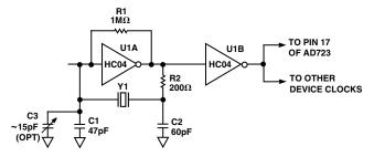
Figure 9. Low Cost Crystal Oscillator
