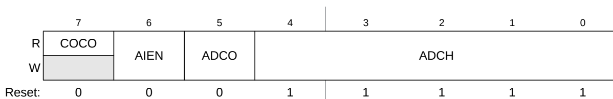
Figure 10-3. Status and Control Register (ADCSC1)
