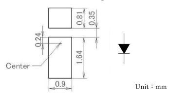
Mountability and solderability need to be optimized with actual conditions such as amount of solder, reflow temperature applied in the process.
