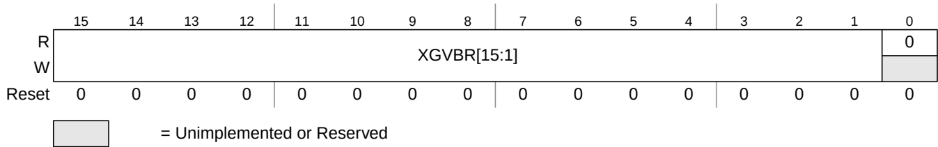
Figure 5-5. XGATE Vector Base Address Register (XGVBR)
