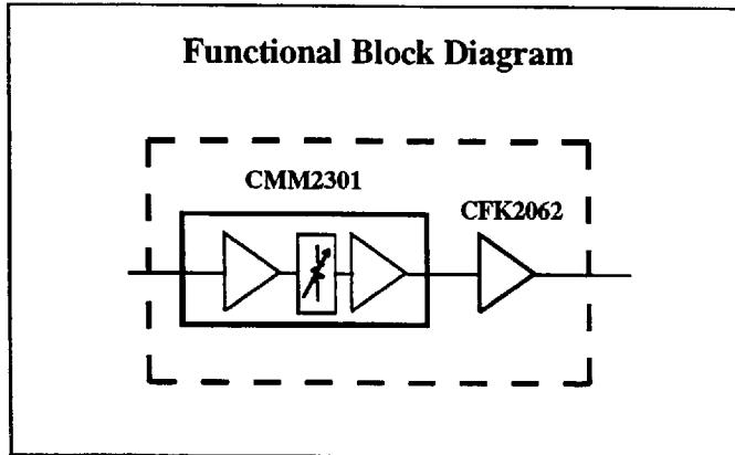
analog level adjustment capability that allows fine tuning of the output power level over a 10 dB range.
