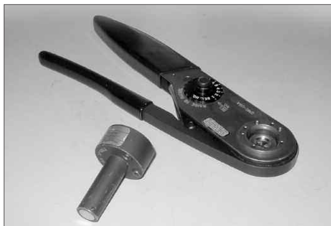
Crimping tool M317 and locator VGE1 0077A
